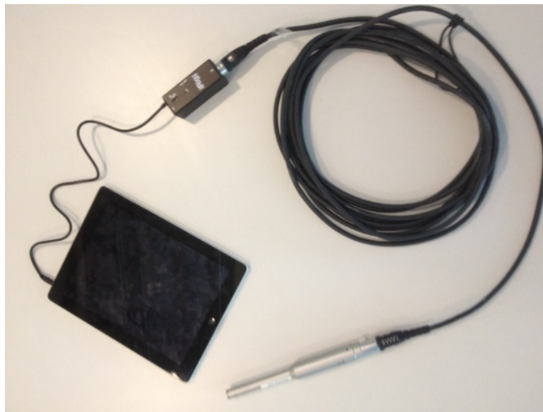
Figure 1: Microphone setup for an iPad
